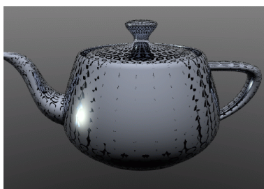
Figure 1.3: Problem of wrong parameters for Newton iteration. Image taken from [MCFS00].
