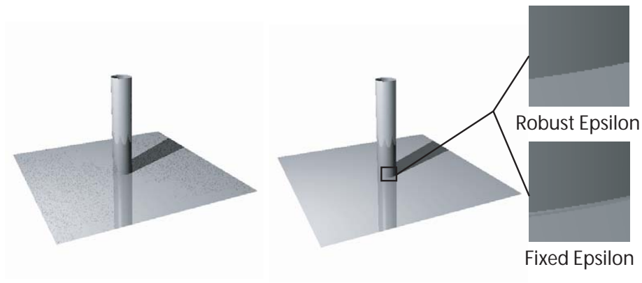
Figure 2.15: The right image shows a scene rendered with shadows and reflection. The left image shows the result without special handling of the point of intersection. The two small images on the right show a closeup of the reflection. When using a fixed epsilon a reflection may start to far away as can be seen in the bottom close up image.
