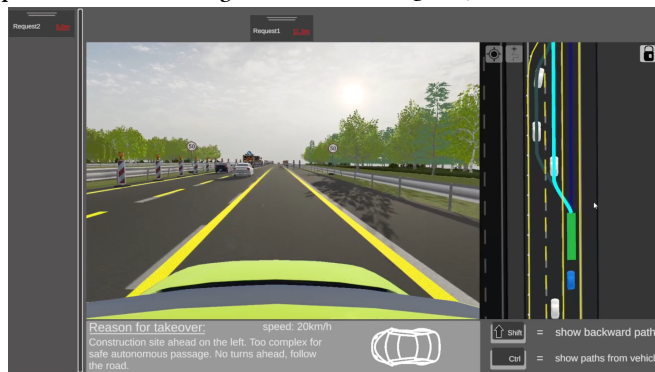
(c) Path planning. Three potential paths are visible and color-coded. A second request is in the queue don't he left.
