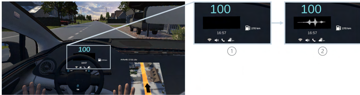
Fig. 3. The inside of the AV with the control functions at the steering wheel. (1) shows the display without speech output and (2) shows the speech wave animation displayed during AV speech output. For the animation, we used a video by Vecteezy .
