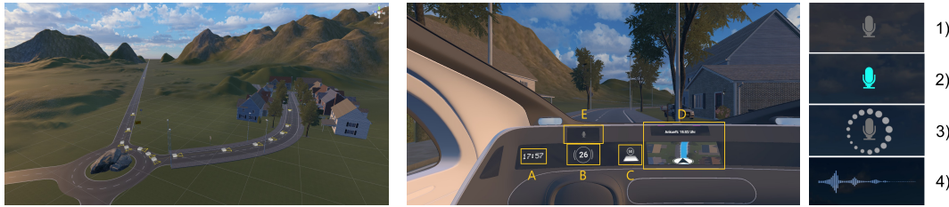
Fig. 3. Participant’s point of view (left). On the AV’s dashboard, there is a clock (A), the current speed (B), the registered speed limit (C), and a navigation system (D) that shows directions and arrival time. Also, the AV’s voice assistant has a separate display (E) that indicates its current status (right): 1) inactive, 2) active and listening, 3) transcribing/ loading, and 4) speaking. The loading icon rotates around the microphone while the assistant processes the voice input and generates its output.
