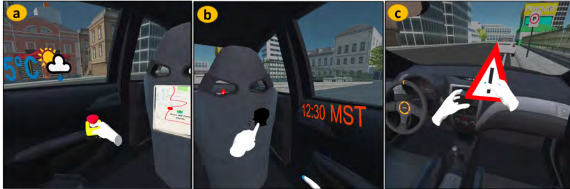
Fig. 1. AV-Sketch Interfaces: (a) a participant is manipulating 3D objects- stop button, visual display, weather/time icons in the VR scene (P5), (b) a participant is selecting auditory cues (P3), and (c) a participant is designing interfaces for the critical road scenarios with a warning symbol and placing the 3D element near the dashboard using the 'grab' feature of Quest hand tracking (P2).
